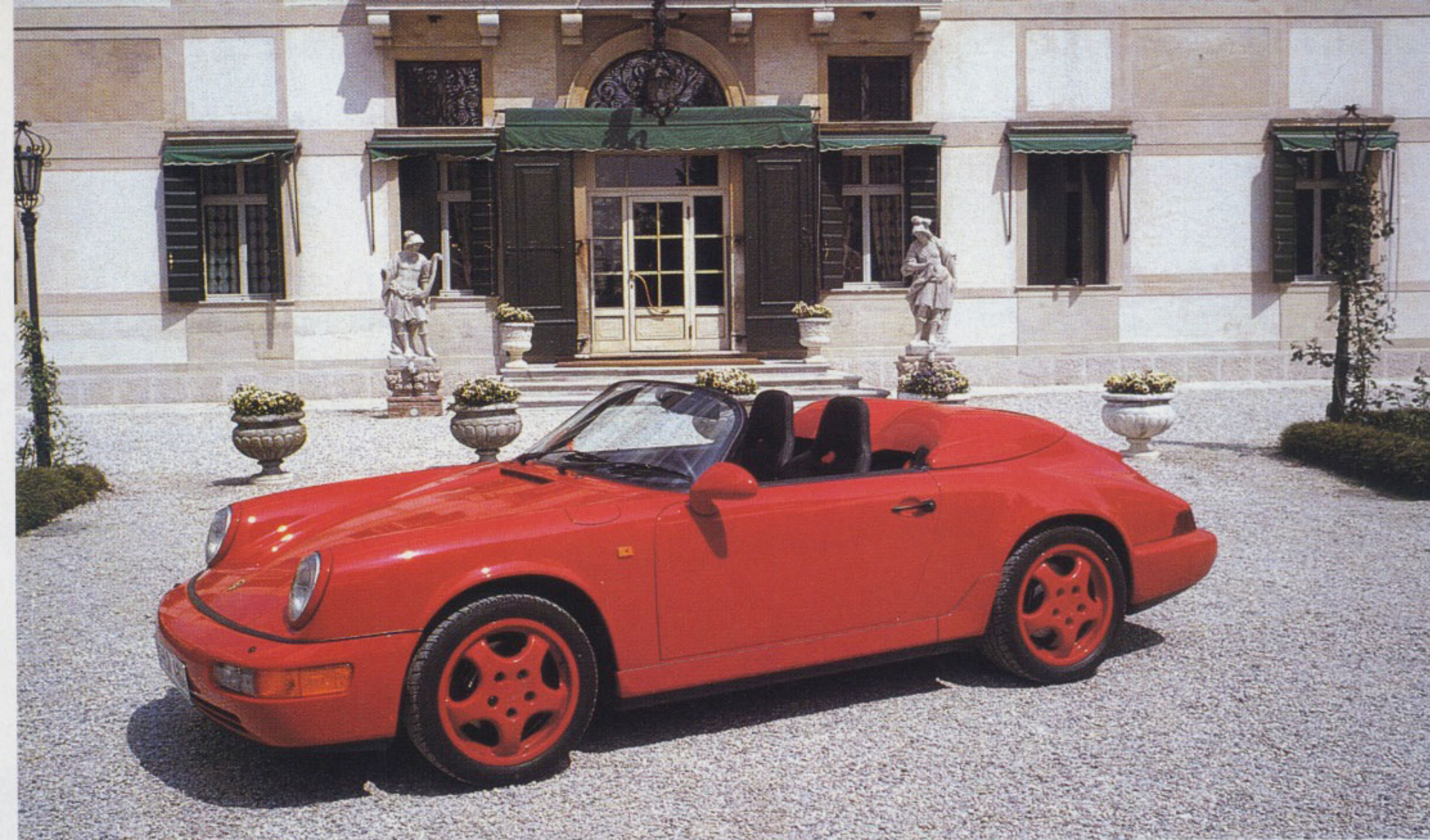
Three-quarter view reveals the twin-hump rear lid to cover the folded top — a Speedster feature since the 1987-89 version.
